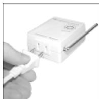
3. Plug the Transceiver Module into a convenient AC outlet. Fully extend the antenna.
