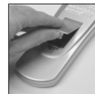
2. Fit four AAA batteries, taking care to match the + and - marks in the battery compartment.
