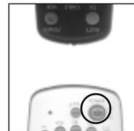
6. Press the button on your existing remote that you want to learn. Hold the button until the LED on the UR74A Remote blinks off.
