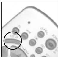
4. To find the first digit, press each number button from 0 to 9 until the LED blinks. The number you pressed is the first digit of the code.
