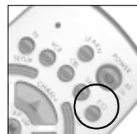
3. Enter 998 to control an IR Mini Controller, or 999 for standard X10 control. The LED turns off after the last digit entered.
