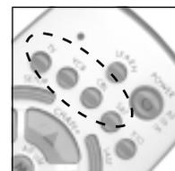
4. Press CHANNEL + repeatedly (note 5, page 12) until the device to be controlled changes channel.
