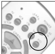
2. Press and hold SETUP until the LED indicator lights steadily. Release Setup button.
