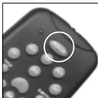
6. Turn your device on and press CHANNEL+. If the device responds, setup is complete.
