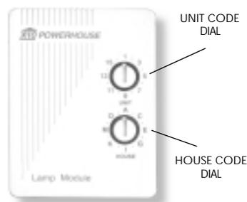
Each Module has a specific address made up of a House Code (red dial on the face of the Module) and a Unit Code (black dial on the face of the Module).
