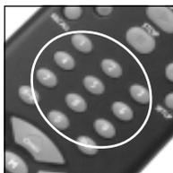
Once in X10 mode you can control any X10 Module by pressing the number button corresponding to its Unit Code, followed by the appropriate function key as follows:
