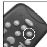
4. Press and release the mode button that matches the A/V equipment you want to control. The LED blinks once.
