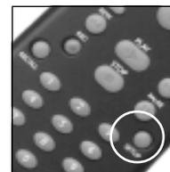
3. Press and release the mode button that matches the device you want to control. The LED blinks once. Use AUX for CD equipment.
