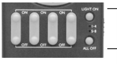
The Lights On button turns on ALL lights connected to Lamp Modules and Wall Switch Modules (set to the same Housecode as the remote). This button does not affect Appliance Modules.
