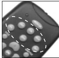
4. Press CHANNEL + repeatedly\*\* until the device to be controlled changes channel.
