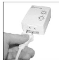
3. Plug the Lamp Module into a convenient AC outlet.
