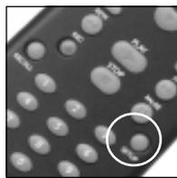
3. Press the mode button\* that matches the equipment you want to control. The LED blinks once.
