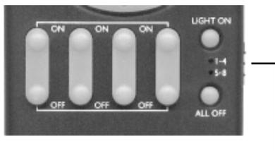
Use the slide switch on the side of the remote to select control of X10 Modules set to 1-4 or 5-8.
