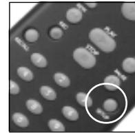
4. To find the first digit, press each number button from 0 to 9 until the LED blinks. The number that blinked is the first digit of the code.
